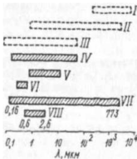
Fig. 4. Diagrams of lasing wavelengths overlapped by active lasers: I is the possible region of lasing at rotational transitions; II - possible region of generation on vibrational-rotational transitions; III—possible region of generation on electronic transitions; IV - semiconductor lasers; V—chemical lasers; VI, dye lasers; VII - gas lasers; VIII - solid state lasers
