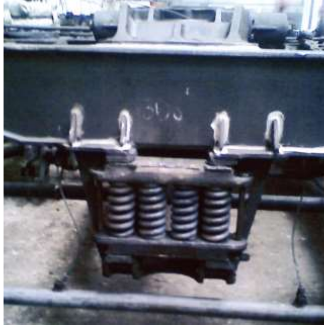
Figure 1. Appearance of support unit (support) of traction electric motor NB-418K with support-axis suspension for electric rolling stock VL-80s in the form of a system of parallel spiral cylindrical springs
