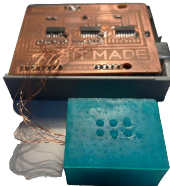
Figure-9. Connecting process of a single-cell display unit and a control unit of the proposed display
