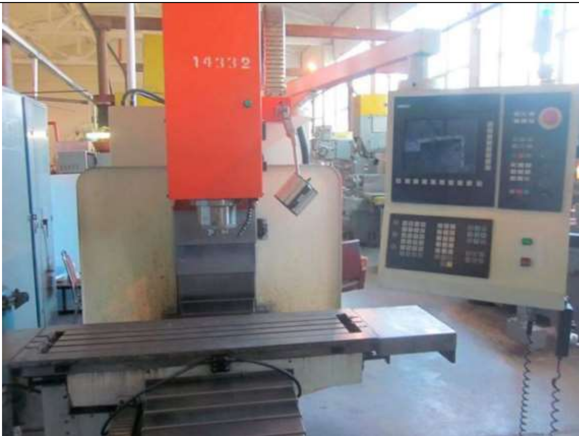
Figure 2.28. Vertical milling machine with CNC 6B52F3.
